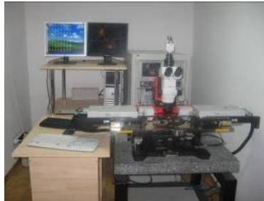
The millimetre wave characterization equipment up to 110 GHz
