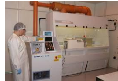
The Au plating facility for semiconductor wafers
